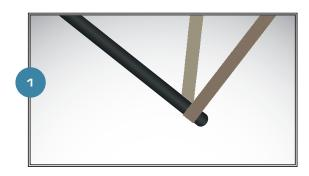
Shaft should be sanded to the top of sleeve to get maximum grip.
