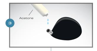
Dry fit sleeve into hosel to ensure correct depth and clean both hosel and sleeve thoroughly with acetone.
