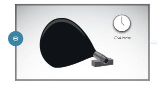
Lay the clubhead on its side to dry and support the neck so that the hosel is horizontal. This will both prevent any epoxy from running into the hosel cavity, and also stop the sleeve from slipping back while the epoxy cures.
