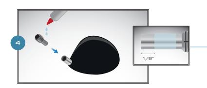
Apply good quality long-set [24 hour] epoxy to the body of the SLEEVE ONLY. It is very important that there is no surplus epoxy on the inside of the sleeve so only apply enough epoxy to cover the surface of the sleeve and leave appropriately 1/8" clean at the tip of the sleeve.
