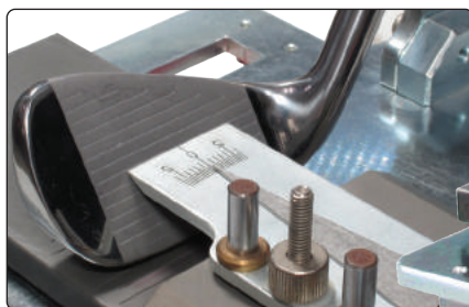
▲ The apron and base provide two reference planes from which an accurate setup can be achieved.
